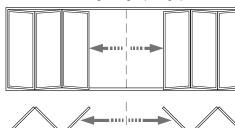
Choose to fold Visofold doors internally or externally.
